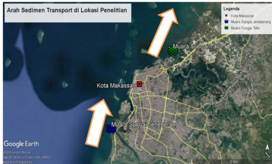
Figure 4. Longshore sediment transport directions in the Tallo river estuary and the Jeneberang river estuary towards the Makassar coast
